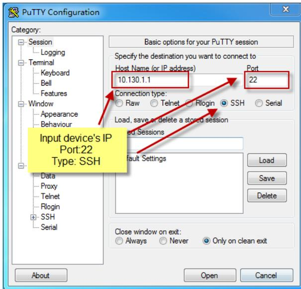
IP address: IP address of LG01-N
