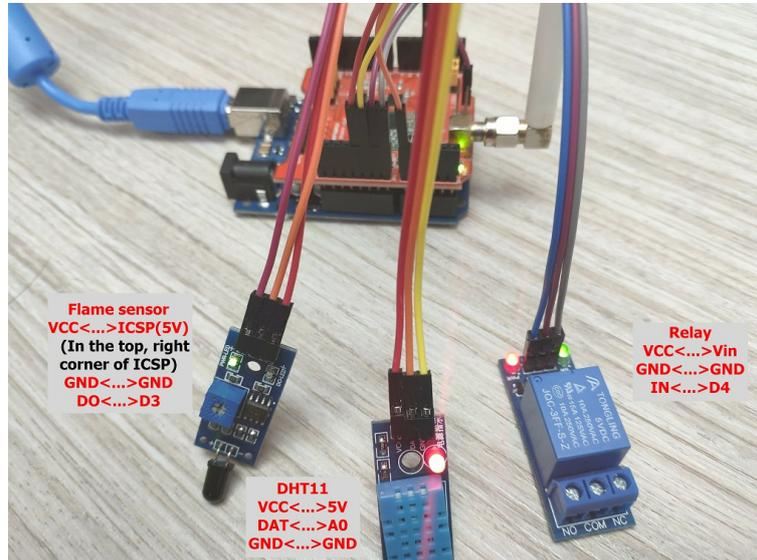
There are three sensors connect to the LoRa Shield + UNO. These sensors are flame sensors, DHT11 (Temperature & Humidity sensor) and Relay. Please use the connection as we show in the photo.
