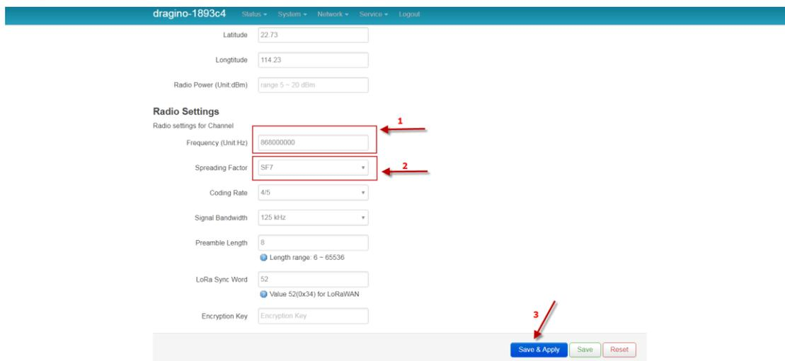
The screenshot shows the web interface for configuring a channel. The top navigation bar includes 'dragino-1893c4', 'Status', 'System', 'Network', 'Service', and 'Logout'. Below this, there are input fields for 'Latitude' (22.73), 'Longitude' (114.23), and 'Radio Power (Unit: dBm)' (range 5 - 20 dBm). The 'Radio Settings' section is titled 'Radio settings for Channel' and contains the following fields:
