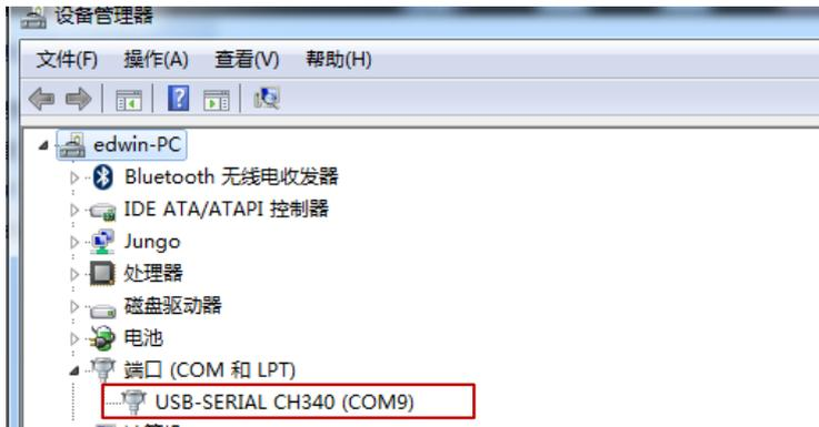
After install the driver, start Arduino and we will be able to use the board Arduino UNO and corresponding COM port to program UNO now.
