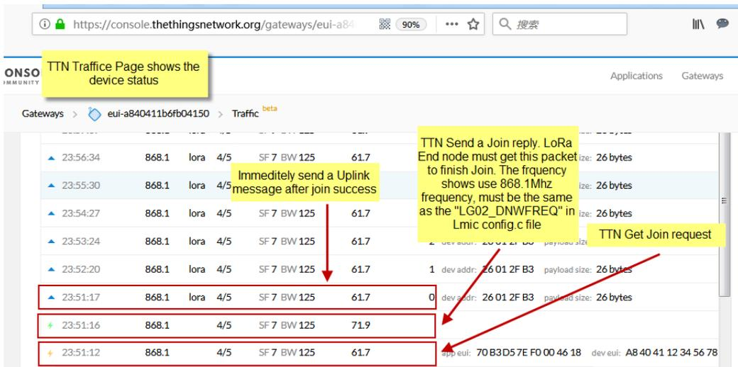
Note: The LG02\_DNWFREQ value in Arduino\_LMIC/src/lmic/config.h should match downlink frequency from TTN.
